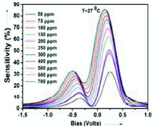
**Fig. 6.** Sensitivity vs bias voltage for various concentrations at room temperature at  $f = 25$  KHz.
