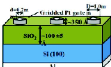
Fig. 1. 3D structure of gridded Pt gate MOS sensor<sup>14</sup>.
