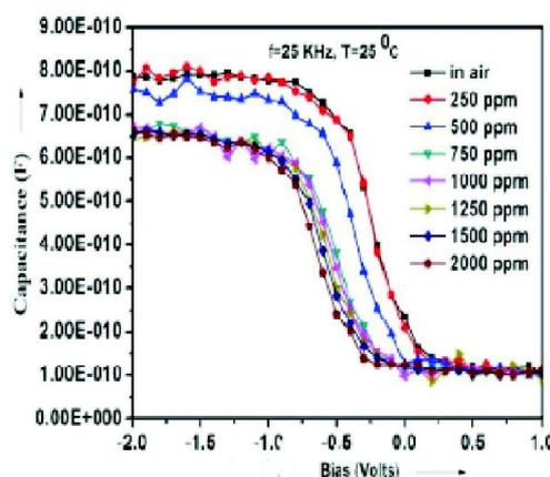
Fig. 3. Capacitance vs voltage (C-V) response of Pt gate MOS sensor at various concentration of H<sub>2</sub> at room temperature at  $f = 25$  KHz.
