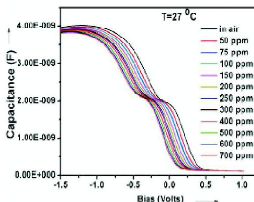
Fig. 4. Capacitance vs voltage (C-V) response of Pt gate MOS sensor at various concentration of NH<sub>3</sub> at room temperature at  $f = 25$  KHz.
