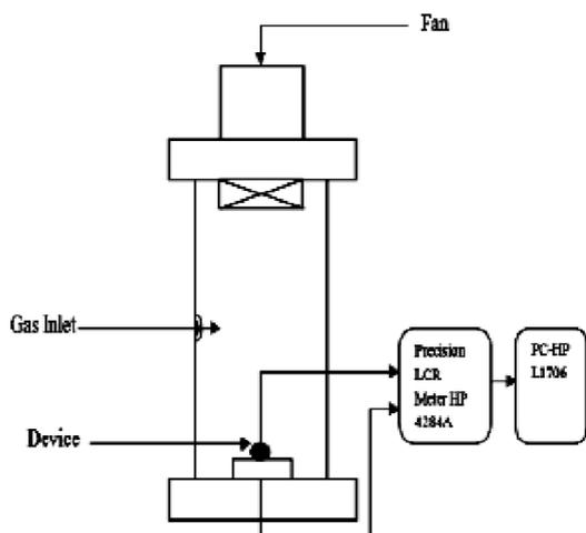
Fig. 2. Experimental setup for C-V measurement of MOS sensor<sup>14</sup>.
